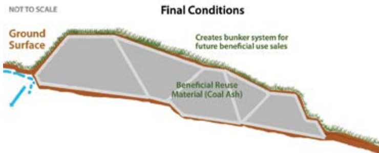
Figure 6 Final conditions, satisfying the beneficial use framework, while creating proper storage for future beneficial use sales. Macroencapsulation on-site clean closure method
